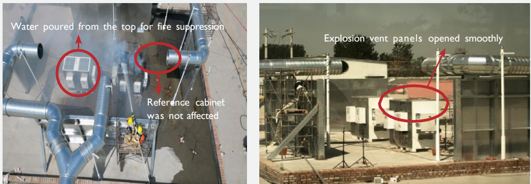
Figure 18. The test result is good, with the surrounding environment well protected Left: image captured by a drone; Right: image captured by a high-speed camera
